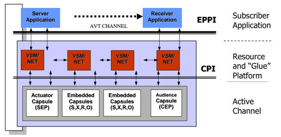
Fig-2 The three-tiers of system architecture in ACF formalism. The top is the subscriber application. It extracts the communication service from the underlying active network via a set of embedded capsules.
