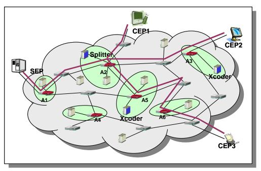
Fig-8. The base topology between one server and three players. Nodes A2, A3 A5 maps one splitter and two transcoders respectively.
