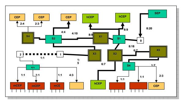
Fig-1 An adaptive video distribution scenario in a network with asymmetric capacities. There are various types of clients. High-definition client (hCEP) have high requirements, and mobile clients (mCEP) delivery. These are also connected with links of different capacities. An distribution network with embedded rate transcoders (X) and stream splitters (S) at correct network points can facilitate the distribution.
