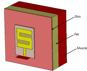
Fig. 2. Three layers model of the human skin designed in CST
