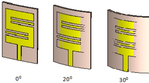
Fig. 3. Different bending angle for the purposed antenna
