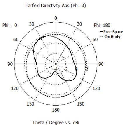
Fig. 9. Simulations of the normalized field patterns in the E plane on free space and on body
