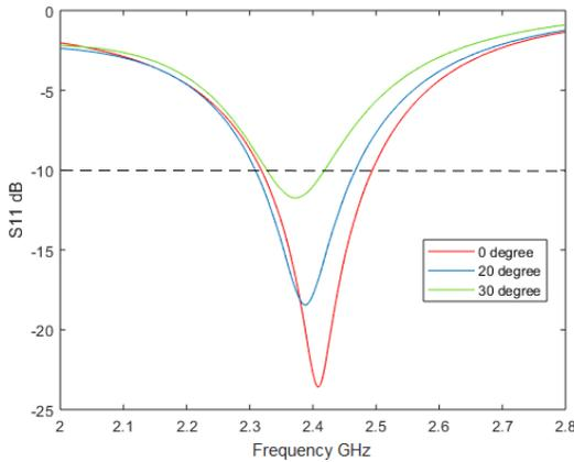
Fig. 4.  $S_{11}$  magnitudes for different bending angles shown in Fig. 3 and without bending
