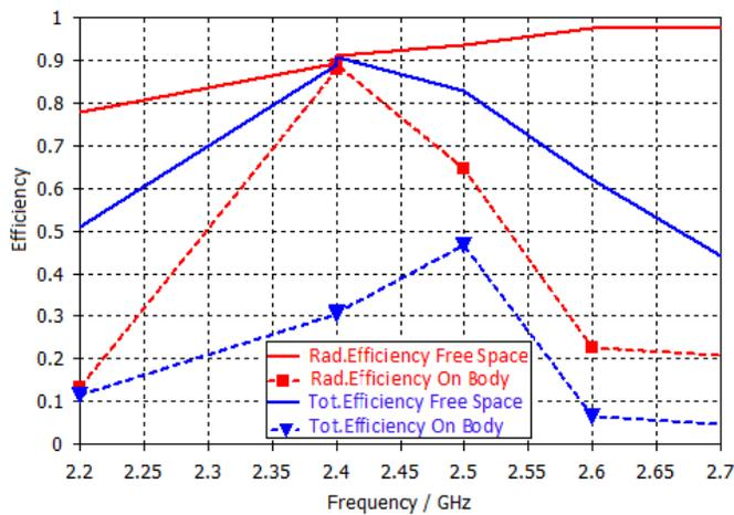
Fig. 7. Efficiency of the antenna on free space and human body
