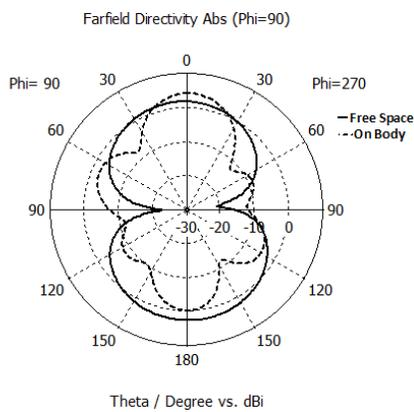
Fig. 8. Simulations of the normalized field patterns in the H plane on free space and on body
