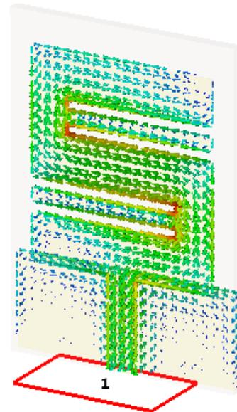
Fig. 6. Surface current distribution of the proposed antenna.
