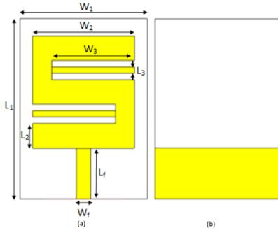
Fig. 1. Patch Antenna with a flexible substrate (a) the front view, (b) the ground plane
