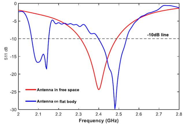
Fig. 5. Simulated  $S_{11}$  profile of antenna for free space and on-body conditions
