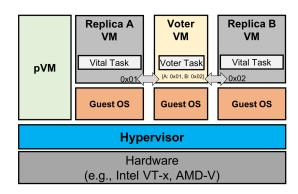
Fig. 2. High-level PoC 2002 architecture.
