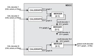
Fig. 2. Multi-Decoder CAL Composer (MDCC).
