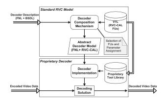
Fig. 1. The RVC design model.
