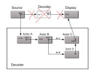
Fig. 6. Substitution of a non atomic node with its correspondent sub-network.
