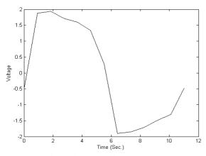
Figure. 2 Waveform of  $x_2$  using 13 points, where M = 6, N = 13, r = 1.5 and T = 11.222s
