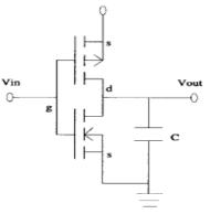
Figure. 5 Schematic of inverter
