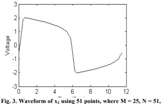
Fig. 3. Waveform of  $x_2$  using 51 points, where M = 25, N = 51, r = 10 and T = 11.589s
