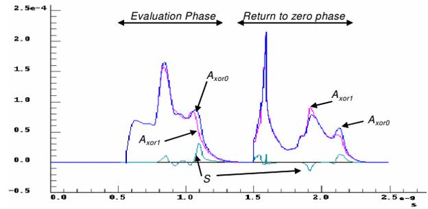
Fig. 6: Electrical signature of a Dual-rail xor gate.
