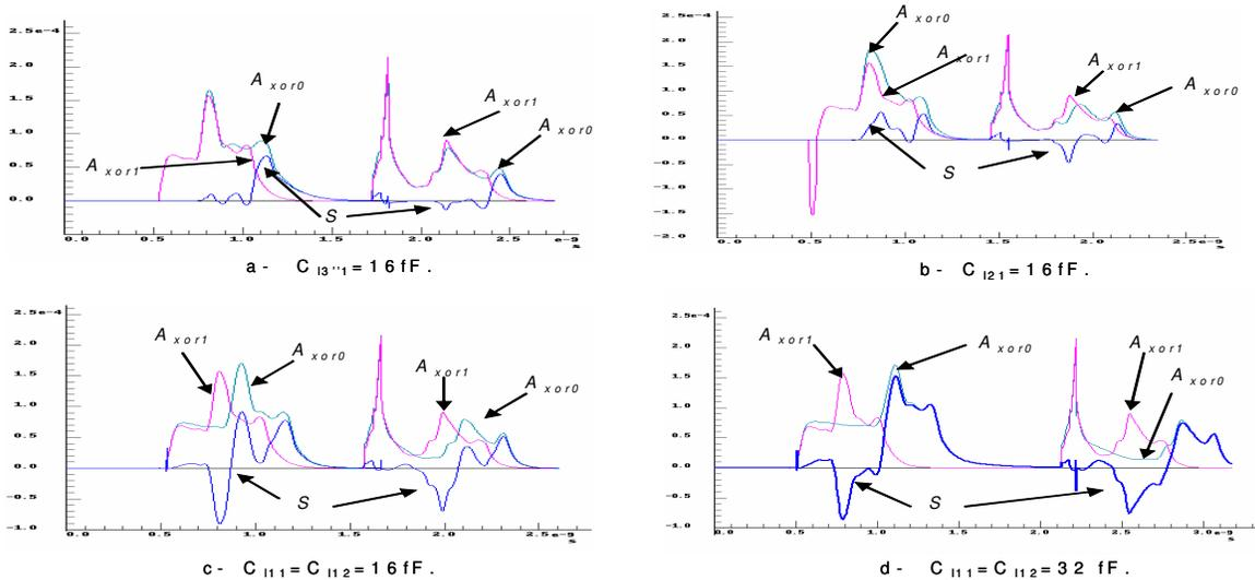
Fig. 7: Electrical Signature of the Dual-Rail Xor gate.
