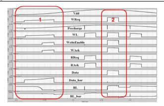
Figure 7. Operatioon of SRAM under varying Vdd
