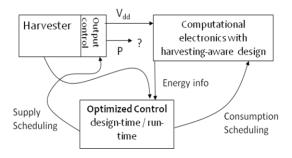
Figure 3. Power-adaptive computing (holistic view)
