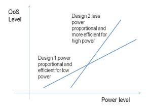
Figure 2. Power-proportional versus power efficient system design
