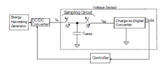
Figure 8. Voltage sensor in an EH-based power chain
