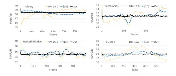
Figure 4: Quality fluctuation of our PQC, conventional [15] and the default HM 16.0 methods. The quality is measured by Y-PSNR. Similar fluctuation results can be found for other encoded video sequences.
