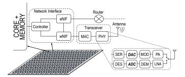
Fig. 2. Schematic of a WNoC architecture with wireless interfaces at the core level. At the transceiver, a generic physical layer module is considered. At the uplink, the transceiver contains a serializer (SER), digital-to-analog converter (DAC), modulator (MOD) and power amplifier (PA). At the downlink, it includes a low-noise amplifier (LNA), demodulator (DEM), analog-to-digital converter (ADC) and deserializer (DES).
