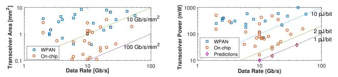
Fig. 3. Area and power of recent transceiver designs for Wireless Personal Area Networks (WPAN) and chip-scale wireless communications, represented as functions of the bitrate. Data extracted from [18], [21] and references therein.
