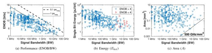
Fig. 4. Snapshot of the historic performance and efficiency of ADCs as functions of the signal bandwidth. Right-side dotted lines delimit WNoC targets.
