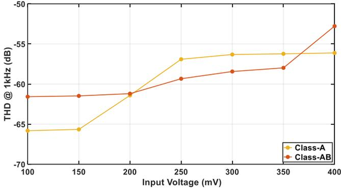
Fig. 8. Measured class-A | class-AB THD vs  $V_{in}$ .
