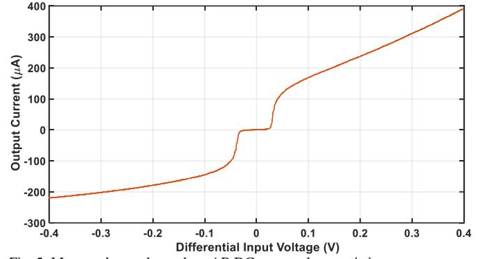
Fig. 5. Measured open-loop class-AB DC output characteristics.
