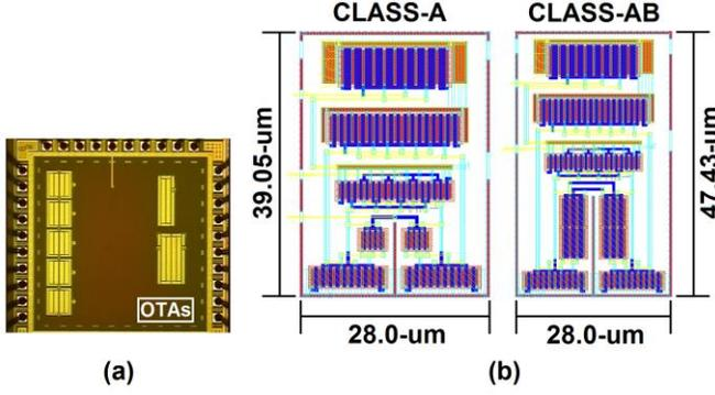
Fig. 4. (a) Test chip microphotograph and (b) OTA layouts.
