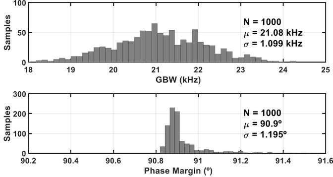
Fig. 9. GBW and phase margin Monte-Carlo analysis for  $V_{DS3} = 50 \text{ mV}$ .
