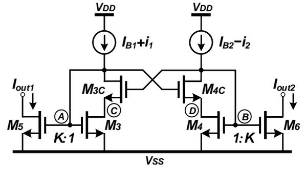
Fig. 3. Non-linear current mirror.
