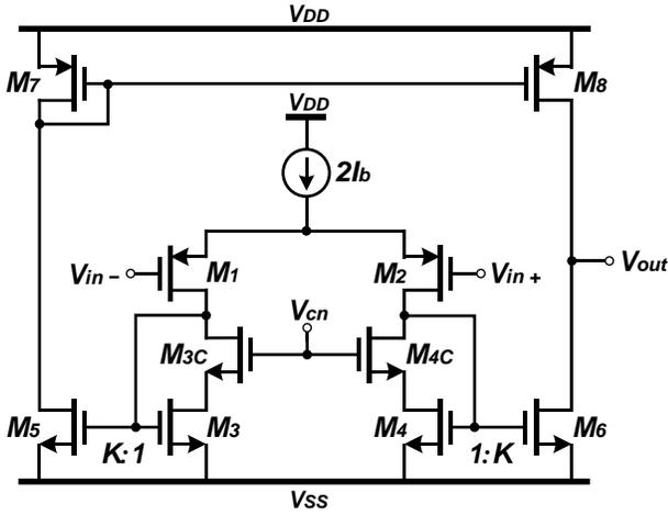
Fig. 1. Conventional single-stage class-A current mirror (CM) OTA.
