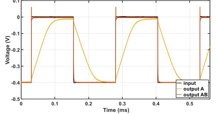
Fig. 6. Measured unity-gain class-A vs class-AB large-signal responses.
