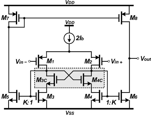
Fig. 2. Proposed class-AB non-linear current mirror (NL-CM) OTA. quantity of devices as in multi-channel processing for large capacitive loads with high-performance slew rates, settling times and power efficiency. A similar approach was independently proposed in [9] without experimental results and published after the circuit design and chip fabrication was carried out by the authors of the present paper.
