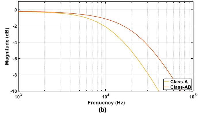
Fig. 7. Measured (a) class-AB open-loop and (b) class-A | class-AB unity-gain closed-loop frequency responses.
