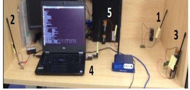
Figure 4: LoRaWAN real network setup with mDots and Multi-tech conduit.
