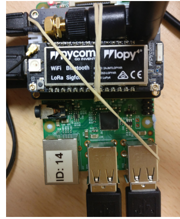
(c) A LoRa gateway connected to a Raspberry Pi serving as the Command Center.
