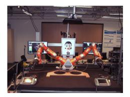
Fig. 1. The FAMULA platform: A bimanual robotic platform supporting the investigation and development of approaches by which a cognitive system can familiarize itself with new objects and concepts through the interplay of manual action and language (https://www.cit-ec.de/en/ deep-familiarization-and-learning).
