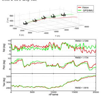
Fig. 5. Results of the take-off stage. The visual estimation (red/dark line) is compared with the GPS/IMU (green/light line) data. As can be seen, the signals have a similar behavior. The normal drift due to the integration is also present. However, its rate is low, allowing to maintain a good approximation of the vehicle's state while the system recovers from a GPS drop-out.
