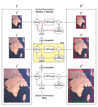
Fig. 1. Multi-Resolution ICIA. Images  ${\bf I}$  and  ${\bf T}$  are downsampled to create the MR structure. In each level, the ICIA is applied iteratively. In each iteration,  ${\bf I}$  is warped, the error between the warped image and  ${\bf T}$  is calculated, and the parameters are updated. When the stopping conditions are reached, the parameters are propagated to the next level. The process is repeated until the lowest level of the pyramid is reached (highest resolution image).
