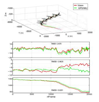
Fig. 7. Results of the landing stage. The visual estimation (red/dark line) is compared with the GPS/IMU (green/light line) data during the landing stage. As can be seen, the signals have a similar behavior, the vision algorithm was able to estimate the vehicle's state until reaching a height of 60 m, and the RMSEs obtained in the attitude estimations are low.
