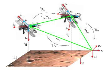
Fig. 2. Pose Estimation based on homographies.
