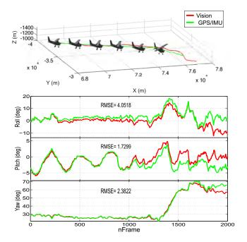
Fig. 6. Results of the cruise stage. The visual estimation (red/dark line) is compared with the GPS/IMU (ligth/dashed line) data. The upper figure corresponds to the 3D position of the vehicle, and the other figures show the estimation of the rotation angles. The errors that were obtained are relatively low considering that the tests correspond to approximately 1 minute of flight.
