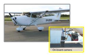
Fig. 3. Airbone System Laboratory (ASL). This laboratory consists of a Cessna 172 equipped with an x86 computer running Linux; a NovAtel SPAN, which computes a tightly-coupled GPS/INS solution for position and attitude data; two cameras: one pointing forwards and the other one pointing downwards; and custom electronics for data synchronization. The ASL is capable of capturing images at a rate of 30 HZ with a resolution of  $1024 \times 768$ .
