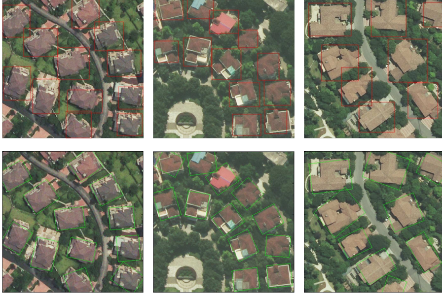
Fig. 7. Detection results comparison between the axis-aligned (upper row) and our proposed method (bottom row).
