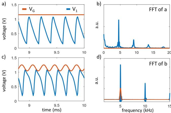
Fig.4: Experimental curves of a single VO<sub>2</sub> oscillator. a) and b) oscillations and corresponding fast Fourier transform (FFT) with a constant gate voltage. c) and d) superimposing an AC signal at the gate voltage, the VO<sub>2</sub> oscillator output signal locks to the AC input frequency, allowing for frequency tuning.
