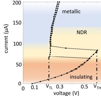
Fig.2: IV characteristic of a VO<sub>2</sub> CB device. The insulating, metallic and NDR regime are highlighted.
