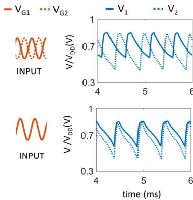
Fig.6: Experimental curves of two oscillator with variable threshold voltage values ( $V_{TH}$  and  $V_{TL}$ ) locked in frequency thanks to the HI synchronization scheme. The relative phase of the oscillators can be controlled through the phase of the AC input.
