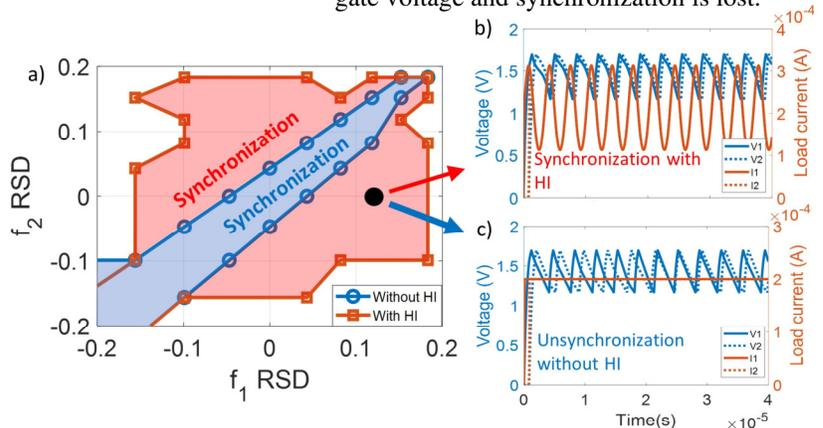
Fig.7: a) Simulations shows the synchronization space of two resistively-coupled VO<sub>2</sub> oscillators with different natural frequencies. Without the HI technique, the synchronization space is limited, with the HI technique synchronization is achieved for diverging natural frequencies up to 18% Relative Standard Deviation (RSD). b) and c) examples of oscillator output with and without HI.
