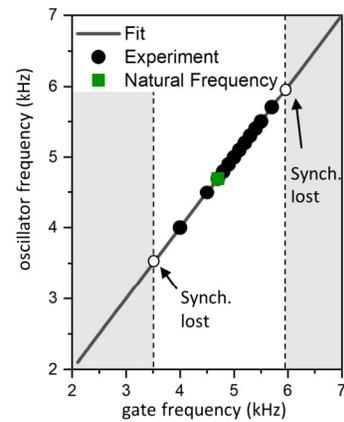
Fig.5: experimental results of frequency injection locking. Changing the frequency of the gate signal, we can tune the oscillator frequency. For  $|f_g - f_n| > 25\% f_n$ , the VO<sub>2</sub> oscillator cannot follow anymore the input gate voltage and synchronization is lost.
