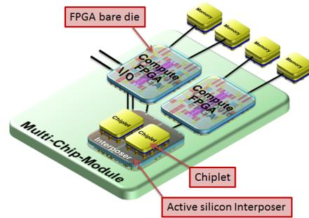
Fig. 3: ExaNoDe Multi-Chip-Module prototype
