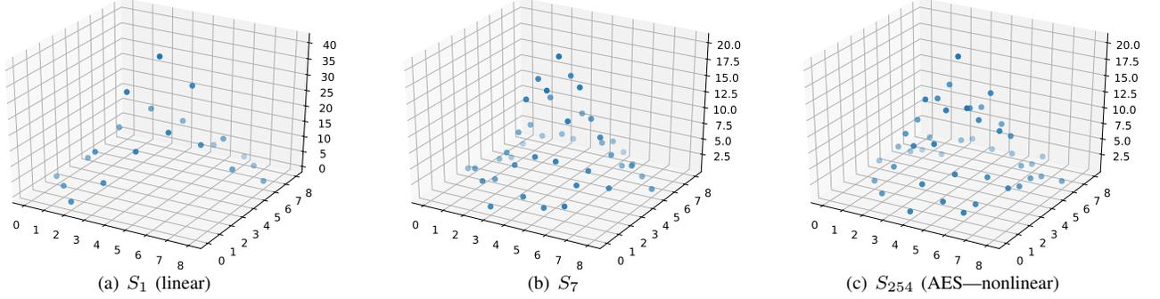
Fig. 3. Number of keys  $M_y$  for given  $Y = y$  for  $t_1 = 0$  and  $t_2 = 3$  for different S-Boxes. The  $x, y$ -axes represent the two coordinates of the 2-dimensional leakage  $Y = y = (y_1, y_2)$ . The  $z$ -axis corresponds to the number  $M_y$  of possible keys given  $Y = y$ , which tends to decrease as the nonlinearity of the S-Box increases. In particular,  $\max_y M_y$  is respectively 40, 20, 20 thereby improving the bound (25) for nonlinear S-Boxes.
