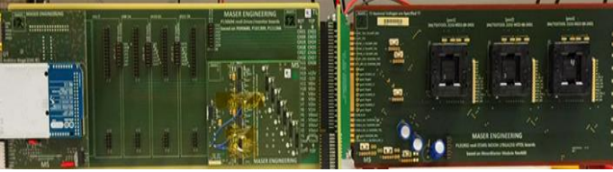
Figure 1. Actual implementation of the accelerated testing system for the Xentium, the cold-zone driver board (left), edge connector (middle) and hot-zone HTOL test board (right) with three DUTs can be recognized. (Courtesy of Maser Engineering).
