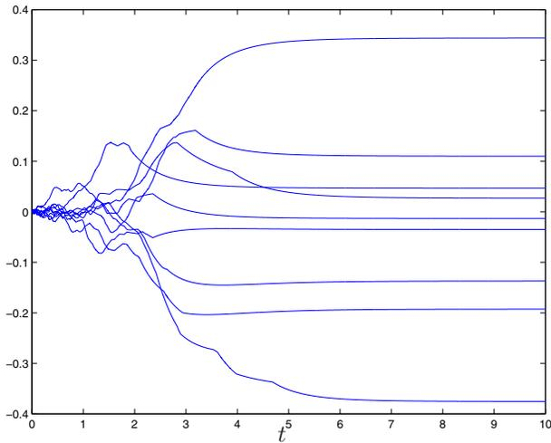
Fig. 5. Sample evolutions of  $\frac{1}{N} \sum_i x_i(t) - \frac{1}{N} \sum_i x_i(0)$  for the dynamics (5) with random initial conditions and  $N = 20$ .
