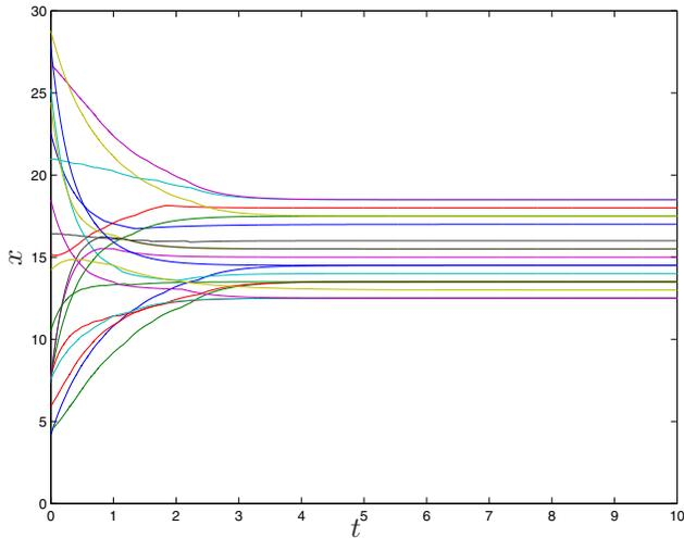
Fig. 6. Simulation of (5) for  $N = 20$  from random initial conditions in  $[0, 30]$ , showing convergence to a non-consensus state.
