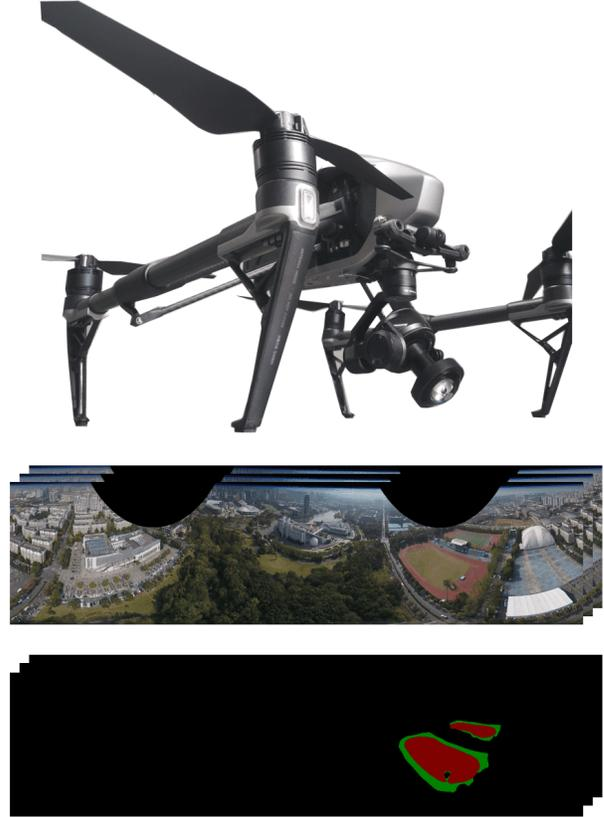
Fig. 1. Overview of our Aerial-PASS system. Panoramic images captured from the UAV with a PAL camera are unfolded, and with the designed semantic segmentation model, field and track classes are predicted at the pixel level.
