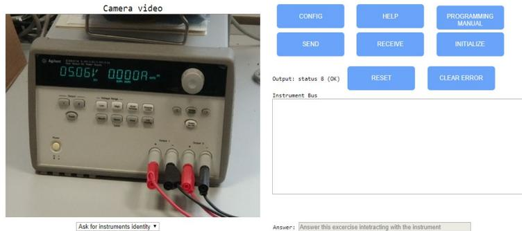
**Fig. 3.** Main web interface GPIB SCPI experience
