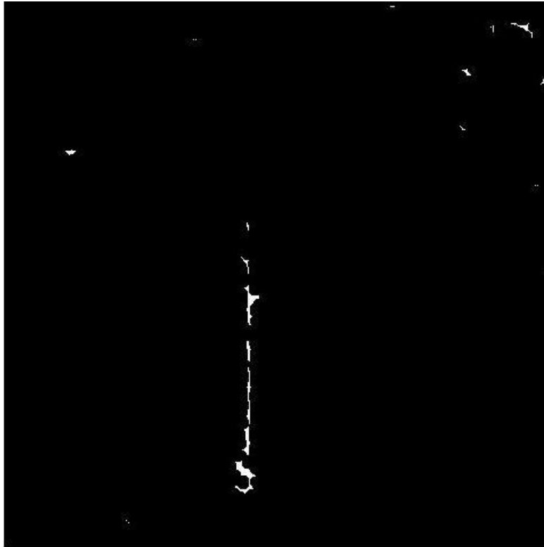
Figure 5-17 A longitudinal crack before connecting
