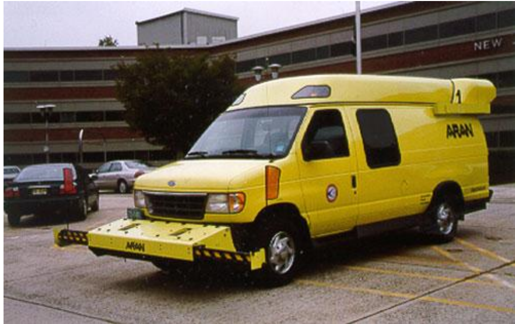
Figure 1-1 Roadware's Automatic Road Analyzer (ARAN)
