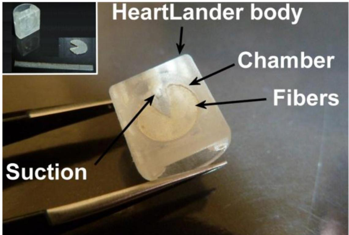
**Figure 5.** Fiber arrangements in HeartLander body; Inset: configurations of laser-cut fibers compared to HearLander body.
