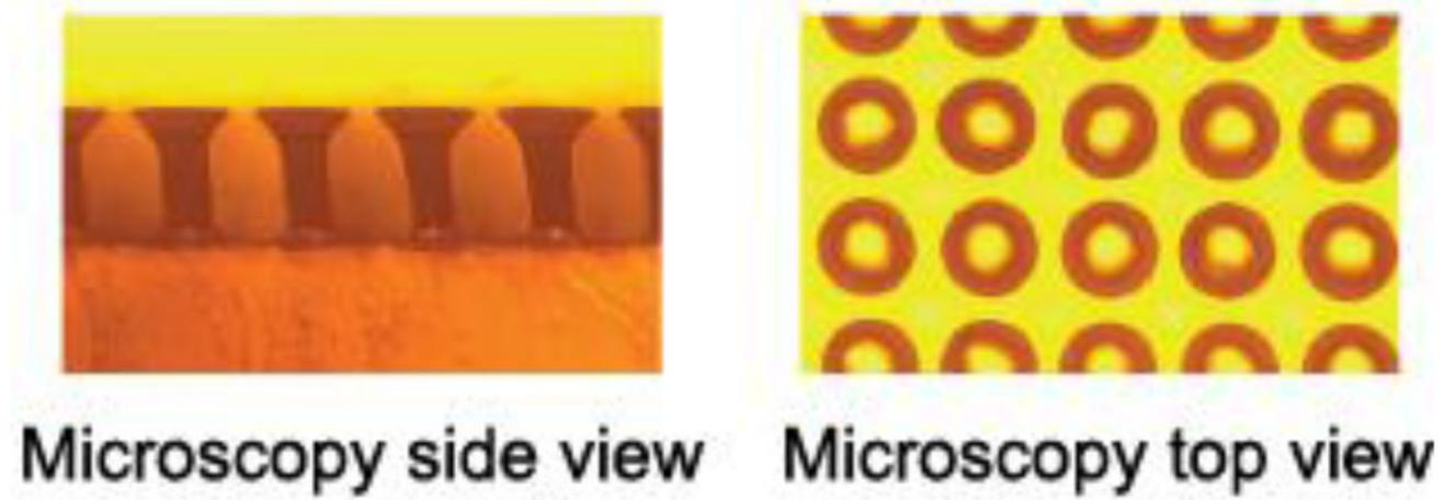
**Figure 2.** Side view and top view optical microscopy images of bioinspired polyurethane fibers. The fibers are 126  $\mu\text{m}$  in height, 42  $\mu\text{m}$  in stalk diameter, and 98  $\mu\text{m}$  in tip diameter.
