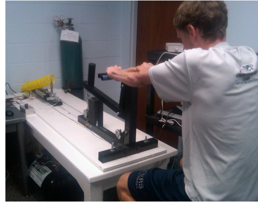
Fig. 6. Demonstration of the hand-forearm ergometer.
