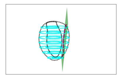
Fig. 2. Schematic diagram of a sample LAX tag plane (green) at ED. As a result of myocardial contraction this plane deforms (not shown) and intersection of the deformed plane with the LAX image plane (black asterisks) will generate a new tag curve (red circles). Endo and epicardial contours extracted from SAX image planes are illustrated by cyan asterisks.
