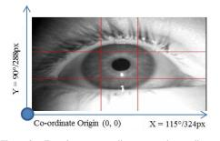
Figure 2. Eye view camera alignment and co-ordinates
