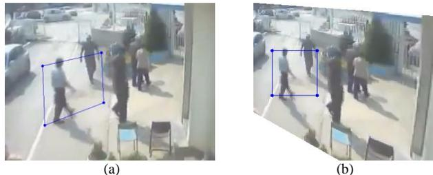
Figure 3. (a) A sample frame showing a person walking from left to right towards the walking hazard; (b) side-view homography of the same image frame (cropped).
