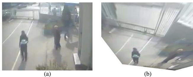
Figure 2. (a) A sample frame showing a person walking from right to left towards the walking hazard; (b) top-view homography of the same image frame (cropped).
