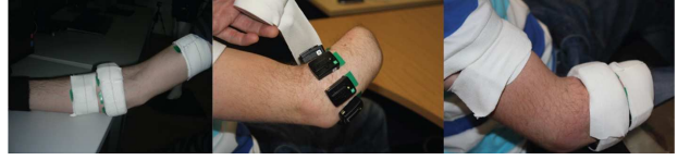
Fig. 1. Sensor placement. Eight EMG-IM sensors were equally spaced around the participants forearm, two targeted the EDC and FDS muscles, and two were placed on the biceps and triceps muscles. Elastic bandage was used to keep sensor positions fixed. Sensor placement shown for an able-bodied (left) and an amputee subject (center, right).
