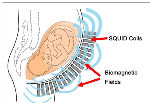
Fig. 1. Schematic drawing of fMEG measurement of biomagnetic signals
