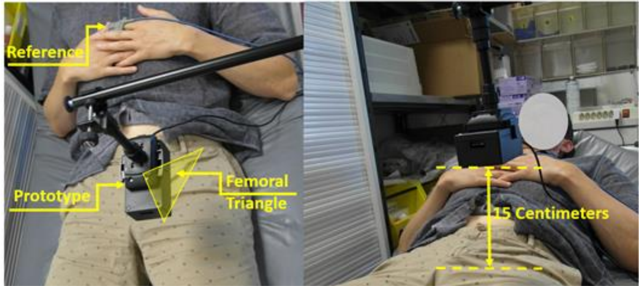
Figure 1. Relative positions of the volunteer and the Doppler radar prototype for contact-less measurement of arterial pulse waves at the femoral region.
