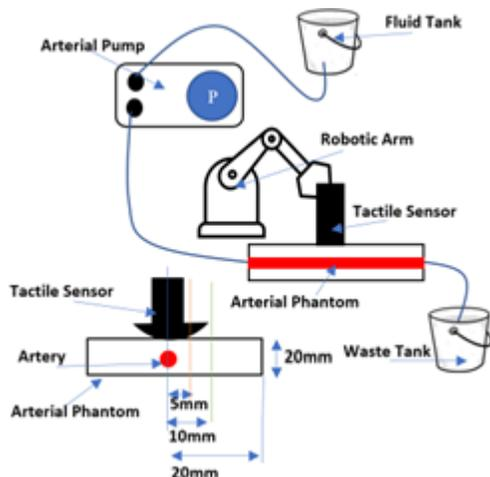
Figure 3 - Experimental Setup Diagram. The tactile sensor is pressed into the phantom in 3 different locations w.r.t. the artery by the robot arm: Centered, 5mm offset, and 10mm misaligned.
