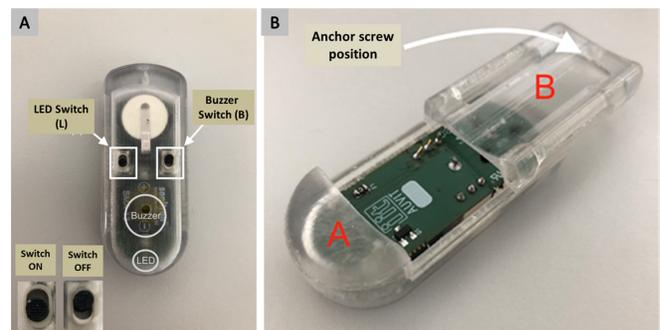
Fig. 2. A. Indication of the switches, B. Opening the device case to allow battery change
