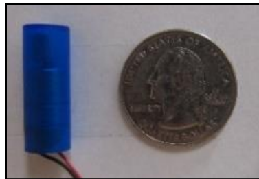
Figure 6. Vibratory motor used for this study. Length: 25 mm. Diameter: 9 mm.
