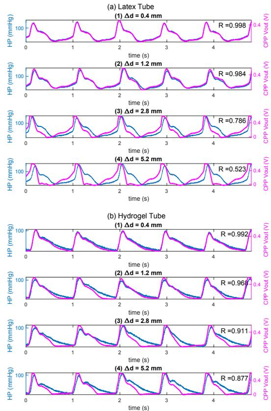
Figure 3. The representative waveform of HP and Cellular PP when (1)  $\Delta d = 0.4$  mm, (2)  $\Delta d = 1.2$  mm, (3)  $\Delta d = 2.8$  mm, and (4)  $\Delta d = 5.2$  mm of (a) latex tube and (b) hydrogel tube.  $\Delta d$  = depression of tube, HP = hydraulic pressure, CPP = Cellular PP, R = correlation coefficient.
