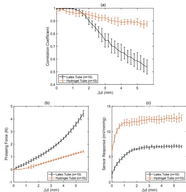
Figure 4. The relationship between depression of the tube ( $\Delta d$ ) and (a) The correlation coefficient between HP (mmHg) and Cellular PP output (V), (b) The pressing force for keeping the depression, and (c) The sensor response (mV/mmHg).
