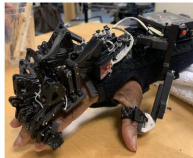
Figure 1. HandSOME II device with magnet activity tracker.
