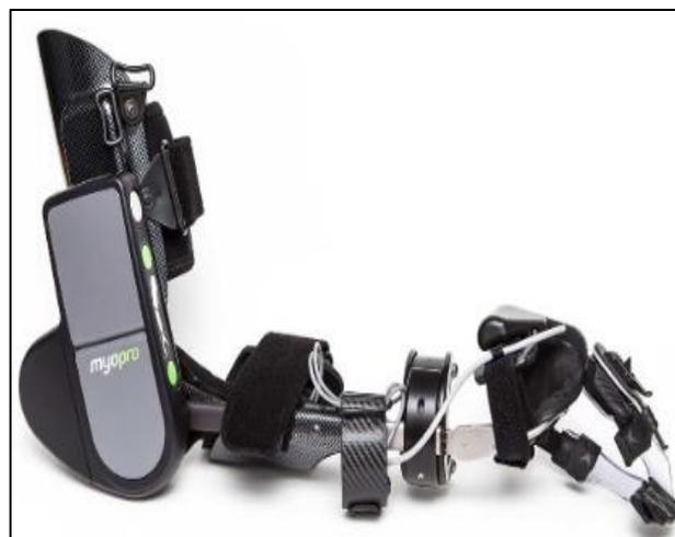
Figure.1. Illustration of the myoelectric upper extremity MvoPro MPWO described in the text
