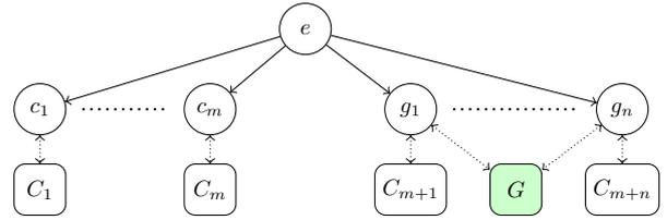
Fig. 2. general deployment setting;  $c_i$  and  $g_i$  represent the  $i$ -th CPU worker and GPU worker, respectively, according the FastFlow numeration of farm workers;  $C_i$  represents the  $i$ -th CPU context according to the OS numeration;  $G$  represents the GPU.
