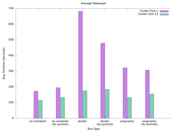
Fig. 4. Average workflow makespan per execution environment setup
