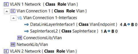
Fig. 14. InstanceHierarchy of the VLAN networks with the respective connection, role and interfaces of VLAN 1
