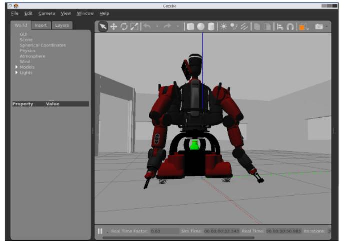
Fig. 4. CS Rack-hosted robot simulation of the Baxter robot with a mobility base
