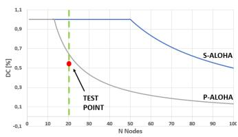
Fig. 5. Maximum Duty Cycle (DC) allowed in comparison with N nodes and channel access methodology
