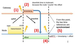
Fig. 4. Synchronization procedure
