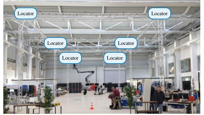
Fig. 1: Experimental setup with six locators in the industrial research campus ARENA2036. The area under investigation spans roughly 20 x 10 meters and the locators are mounted at a height of about 7 meters.
