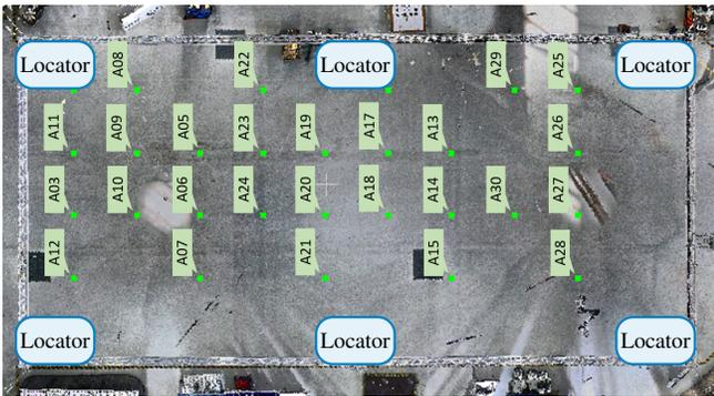
Fig. 3: Top-down view of the area under investigation including the six locators. The positioning accuracy is evaluated at the 28 ground truth points (small green squares).
