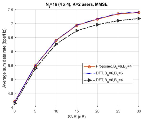
Fig. 5. Comparison on average sum data rate results for  $N_t = 16$  transmit antennas and  $K = 2$  users.
