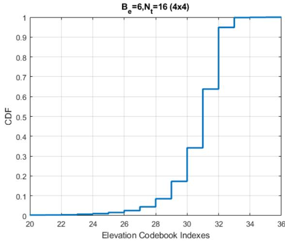
Fig. 1. Distribution of selected codebook indexes in the elevation dimension for  $B_e = 6$ ,  $N_e = 4$  and  $N_a = 4$ .
