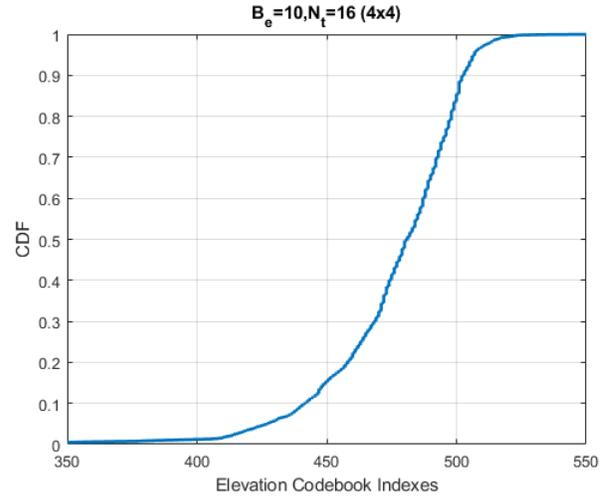
Fig. 2. Distribution of selected codebook indexes in the elevation dimension for  $B_e = 10$ ,  $N_e = 4$  and  $N_a = 4$ .
