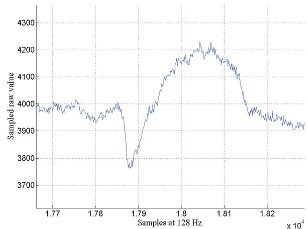
Fig 6. Temporary moving average shift of the EEG data in the timeframe of three seconds
