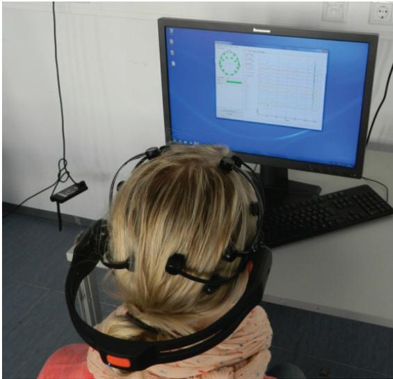
Fig 4. Fitting of the helm to achieve acceptable signal quality was a trial-and-error process which failed in the case of three participants
