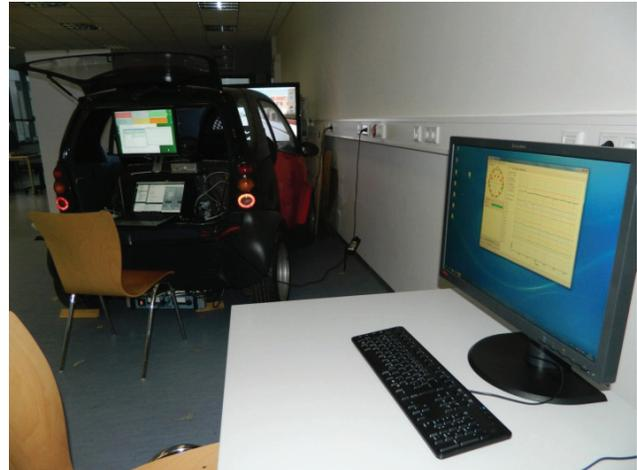
Fig 2. Complete driving simulator setup on the left, personal computer used during helm fitting on the right
