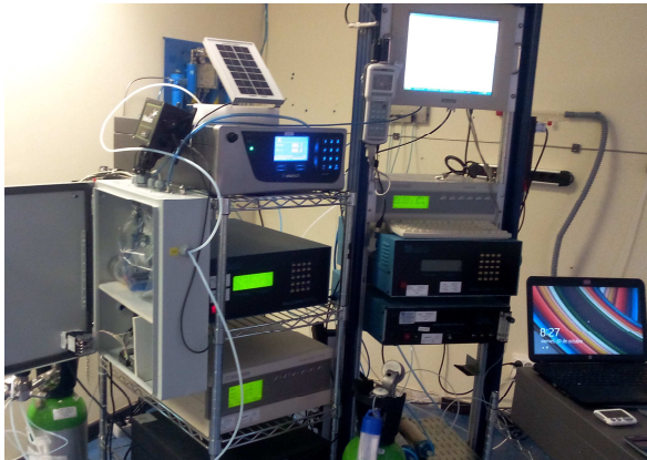
Fig. 1. Complete system for the test of reference gases, relative humidity and temperature
