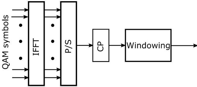
Fig. 2. W-OFDM block diagram.
