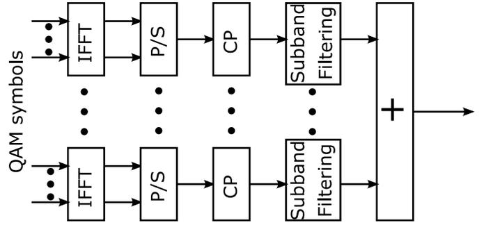
Fig. 3. f-OFDM block diagram.
