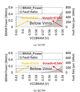
Fig. 3: BRAM Power and Fault Rate Behavior, undervolting below  $V_{min}=0.61V$  until  $V_{crash}=0.54V$ .
