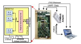
Fig. 1: Undervolting Experimental Setup in FPGA BRAMs.
