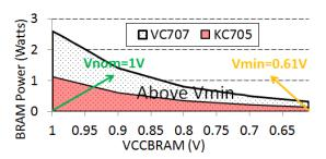
Fig. 2: BRAM Power above  $V_{min} = 0.61V$  in the voltage guardband region (no observable fault).
