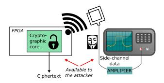
Fig. 7. An illustration of the electromagnetic side-channel attack. The adversary uses electromagnetic-field sensors to capture radiated emissions. To preserve as many frequency components in the spectra as possible, high-quality amplifiers are often used in addition. EM side-channel attack requires physical proximity to the device.
