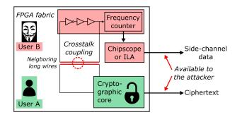
Fig. 5. An illustration of the crosstalk coupling attack. Here, an adversary creates a ring oscillator from an odd number of inverters, one or more buffers, and a long wire. The long wire is chosen carefully, to be very close to another long wire, which is part of the victim. By observing the change in the oscillation frequency of the ring oscillator, the adversary can infer the secret information sent over the victim's long wire.
