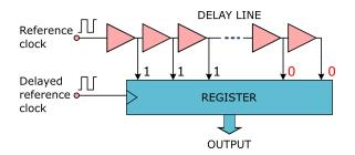
Fig. 2. Simplified architecture of a delay-line sensor. A reference clock signal is connected to a delay line, composed of a uniform chain of buffers. A delayed clock, of the same frequency, is used to sample the propagation delay of the reference clock. Hence, one value is recorded every clock cycle. Since the buffer delay depends on the supply voltage, the output of the register reflects local voltage fluctuations.
