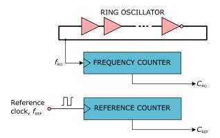
Fig. 3. Simplified architecture of a sensor based on a ring oscillator. The frequency counter keeps track of the number of RO oscillations. The reference counter measures elapsed time. When a fixed-number of reference clock periods expires, frequency counter is disabled and both counters are read to compute frequency  $f_{\rm RO}$ , which reflects voltage variations.
