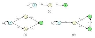
Fig. 3. Freshness of information in (a) a serially connected network, (b) a parallel connected network, and (c) an arbitrarily connected network.
